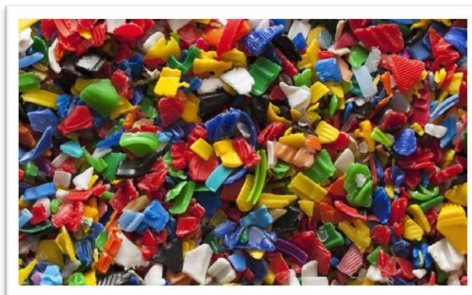
For engineering plastics, Struktol offers multiple products that combine a compatibilizer with lubricants to create a combination product that aids in the incorporation of fillers (mineral or glass) with improved mixing and flow properties as well as mold release. These products result in better processing, improved surface quality, and in some cases, better physical properties.
